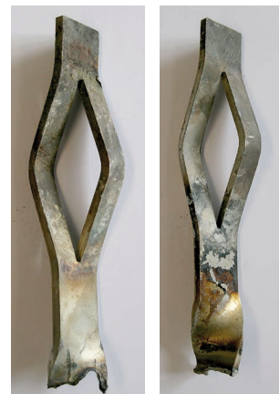
JuSys® ACL anchor after 24,000 operating hours
